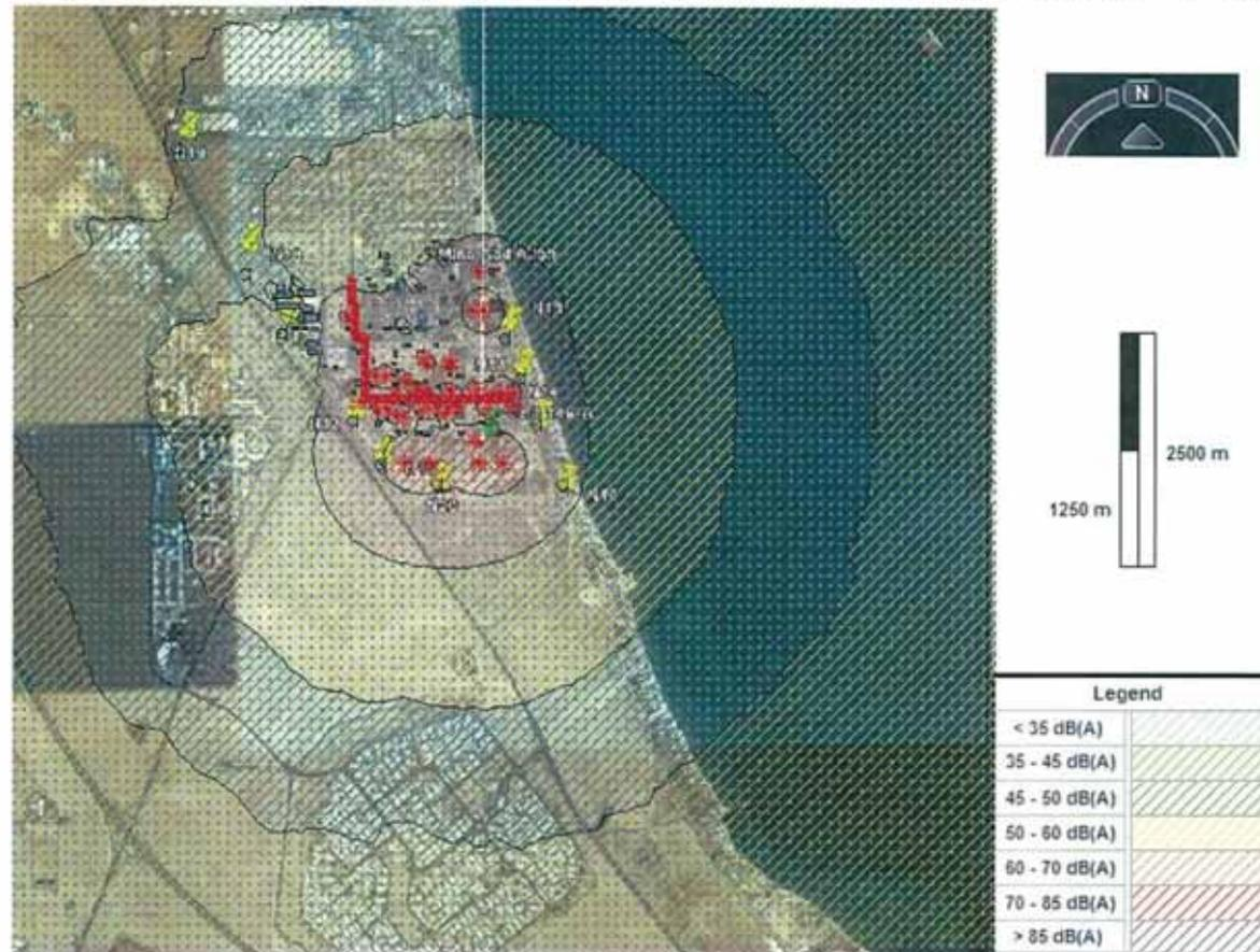
Based on the contour maps shown in Figure 7Q, 7R, 7S, the maximum distances from the fence line of CFP Block in MAB to various noise contour levels are identified as summarised in the following table.
