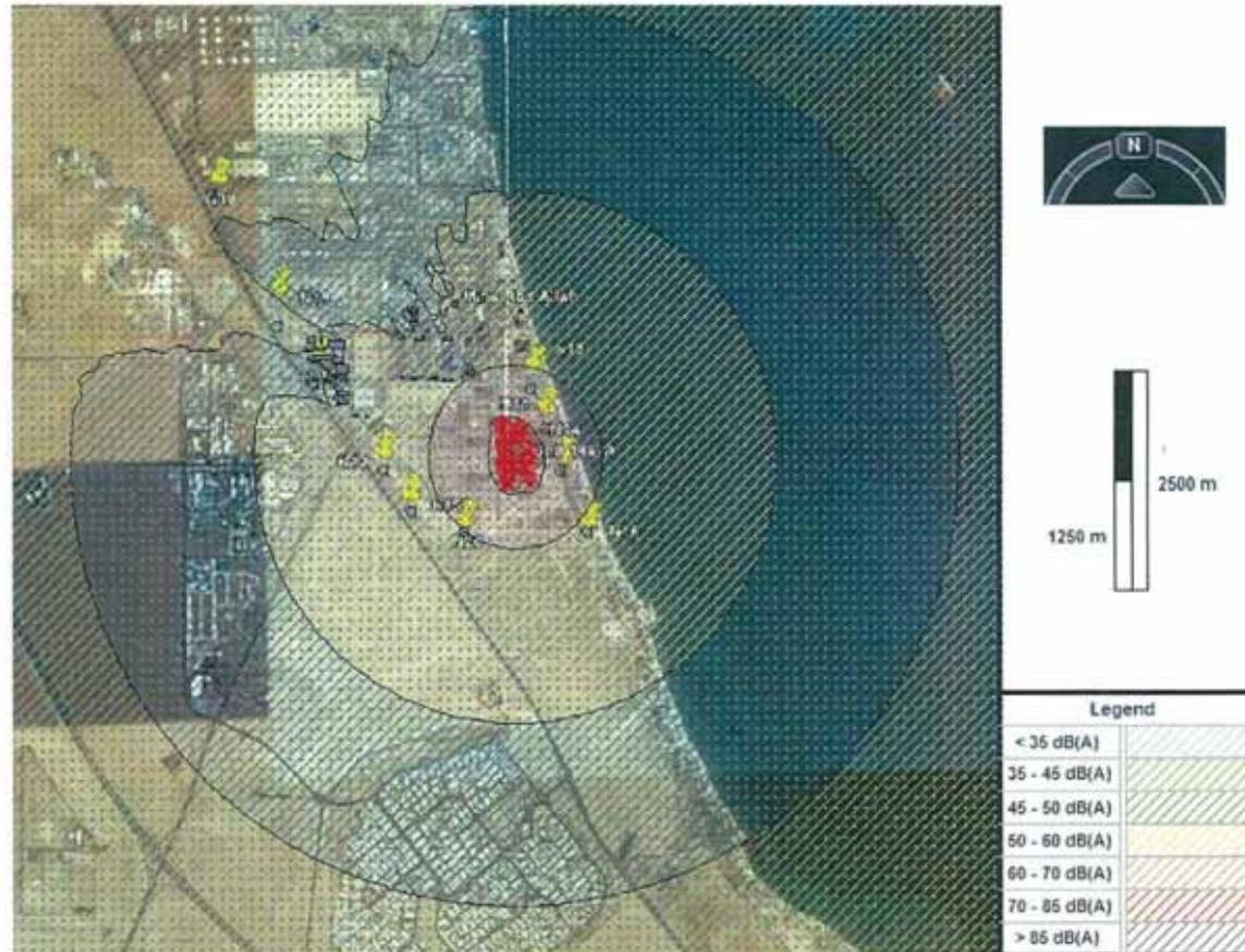
**Figure 7T: Predicted Noise Levels for Operations Phase (Normal Plant Operation) – within MAB CFP Block**
