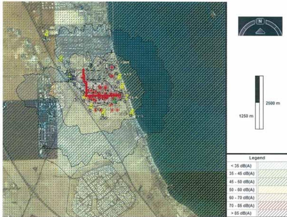
**Figure 7W: Predicted Noise Levels for Operations Phase (Plant Upset Condition) – within MAB CFP Block**
