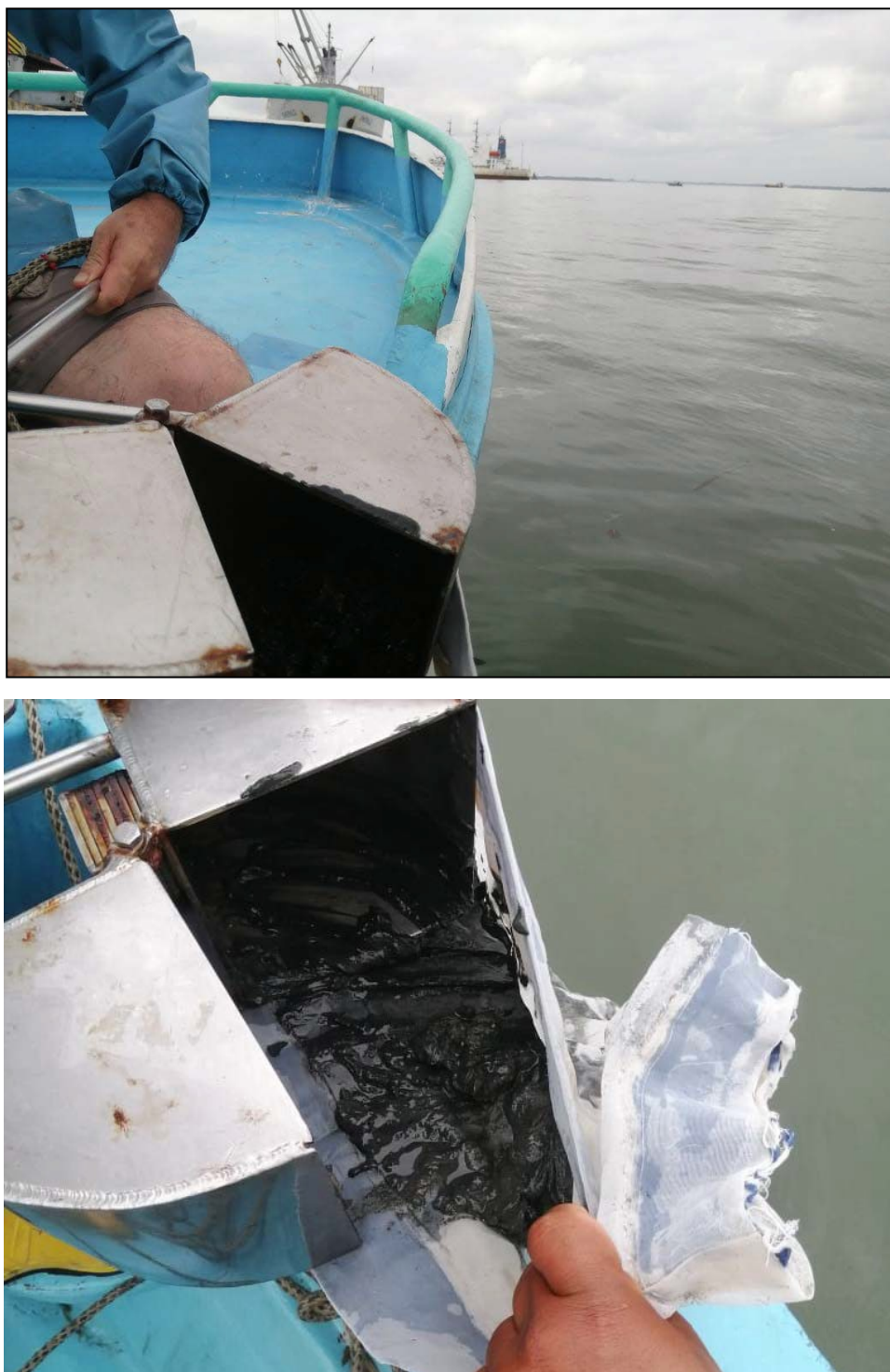
Photographic Record 1. Van Veen Dredge used for Benthic Sampling and Sieving through a 500-Micron Mesh.
