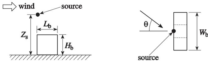
**Figure 2** Parameters of building shape.
