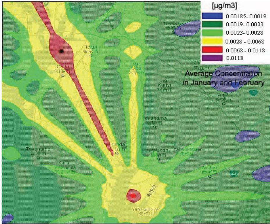
Figure 4. The average concentration distribution of mercury vicinity of two large point sources, calculated with the METI-LIS model in January and February, 2006. The mark of the solid black circle and red circle represents the industrial source locations in the figure.
