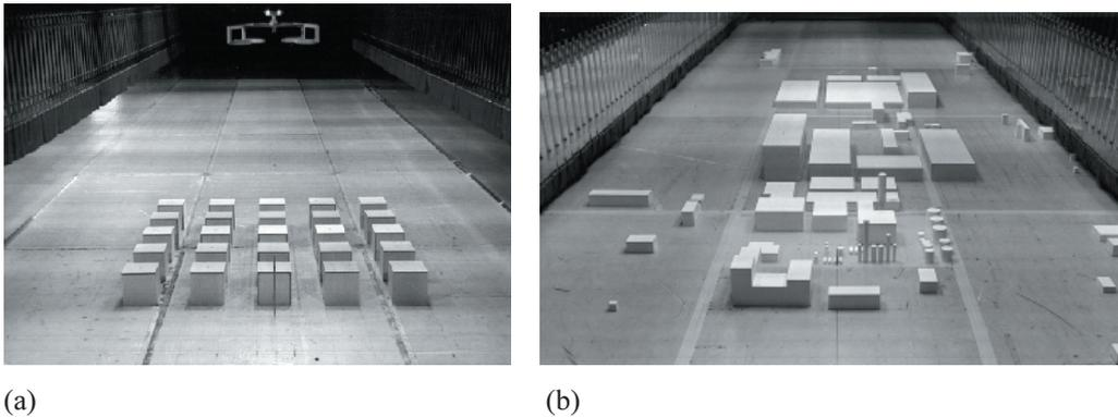
**Figure 3** Examples of scale models used in the experiments: (a) simple-buildings experiments (buildings arrangement  $5 \times 5$ ); (b) factory-buildings experiments.
