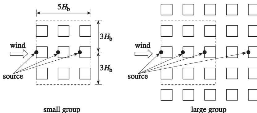
**Figure 8** The method for determination of type of building.
