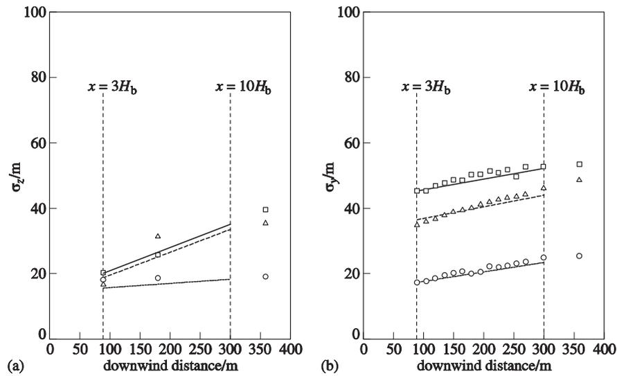
Figure 5 Dispersion parameters: (a) vertical dispersion; (b) lateral dispersion. Symbols show experimental values; lines show the downdraught model.
