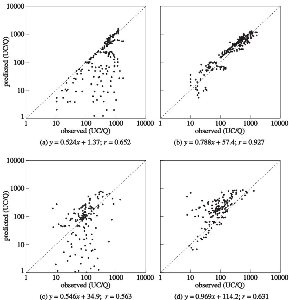
**Figure 10** Comparison between METI-LIS model and original model (wind-tunnel data). (a) ISC vs. simple building experiment ( $5 \times 7$ ,  $Z_s/H_b = 0.5$ ,  $W_b/H_b = 1.0$ ,  $\theta = 0^\circ$ ). (b) METI-LIS vs. simple building experiment ( $5 \times 7$ ,  $Z_s/H_b = 0.5$ ,  $W_b/H_b = 1.0$ ,  $\theta = 0^\circ$ ). (c) ISC vs. factory building experiment. (d) METI-LIS vs. factory building experiment.
