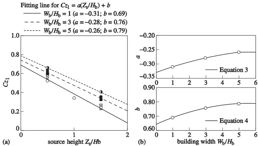
Figure 6 (a)  $Cz_1$  as a function of source height; (b) model of coefficients  $a$  and  $b$ . For  $W_b/H_b = 1$ : number of buildings: ○ = 1; △ = 2; □ = 5 × 5; ▽ = 5 × 7. For  $W_b/H_b = 3$ , ● = 1, ▲ = 2, ■ = 5 × 5.  $W_b/H_b = 5$ , ⊙ = 1).
