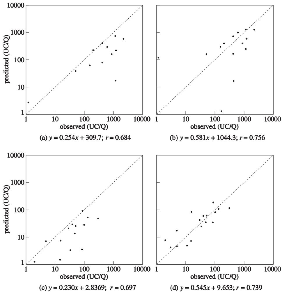
**Figure 11** Comparison between METI-LIS model and original model (field observation): (a) ISC vs. Tsurumi Point (Run 8, 6/7/1971); (b) METI-LIS vs. Tsurumi Point (Run 8, 6/7/1971); (c) ISC vs. Millstone (Run 18, 25/10/1974); (d) METI-LIS vs. Millstone (Run 18, 25/10/1974).
