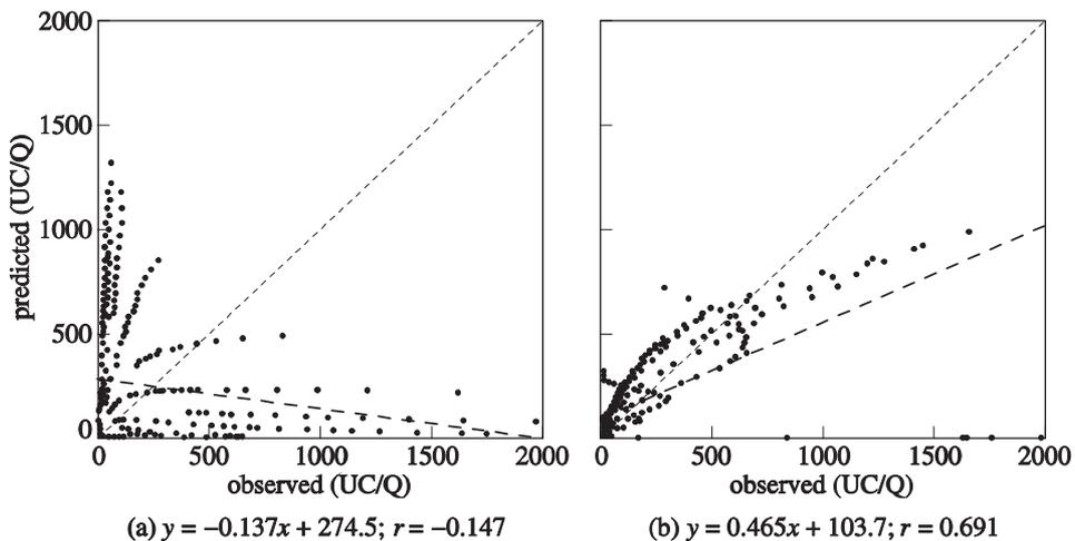
**Figure 7** Effect of source position displacement ( $r$  = correlation factor). (a) Without displacement. (b) With displacement, where  $Z_s/H_b = 0.5$ ,  $W_b/H_b = 3$ ,  $\theta = 20^\circ$ , number of buildings = 1.
