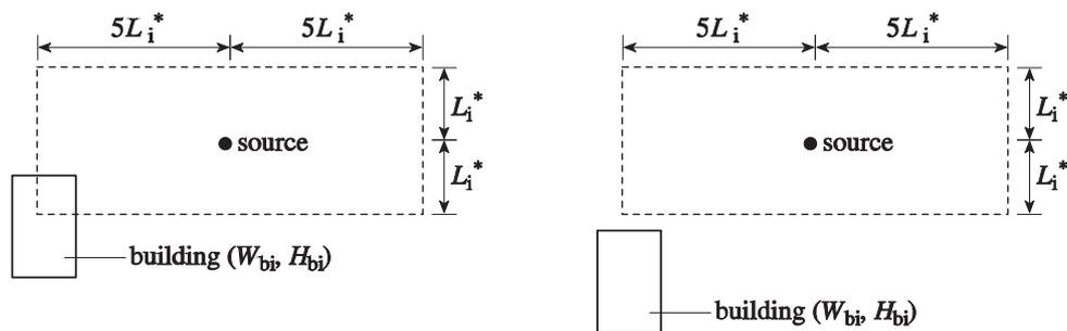
**Figure 9** Determination of the most influential building: (left) with influential building; (right) without influential building.
