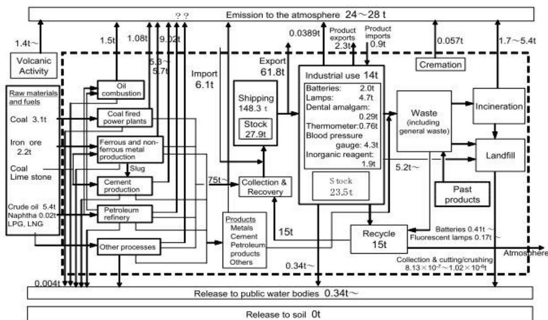
Figure 1. Material flow diagram of mercury in Japan (Kida et al., 2007; Moritomi, 2008).
