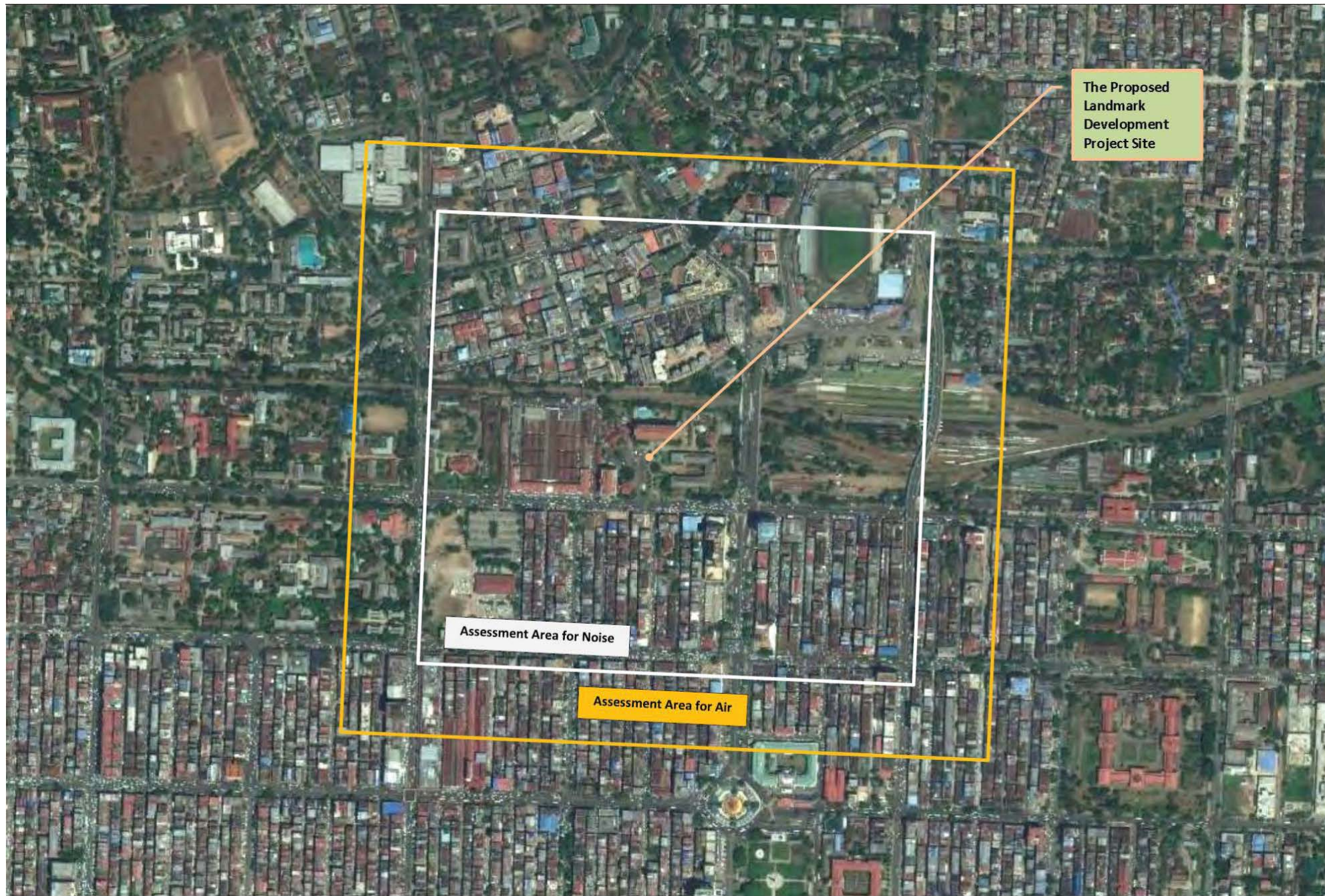
Figure 6.1: Assessment Areas of Air Quality and Noise
