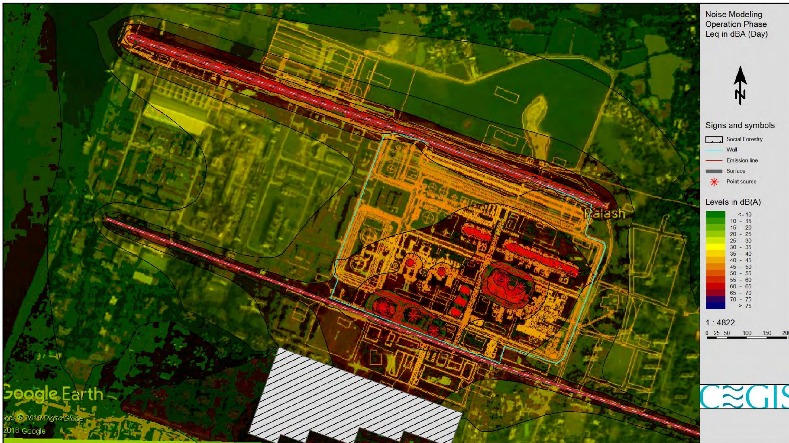
Figure 7.10: Noise Propagation Modeling during Daytime
