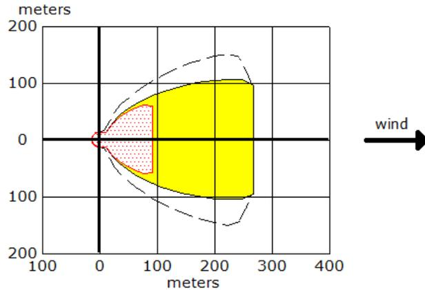
**Figure 10.1: Flammable area of vapour cloud formation**
