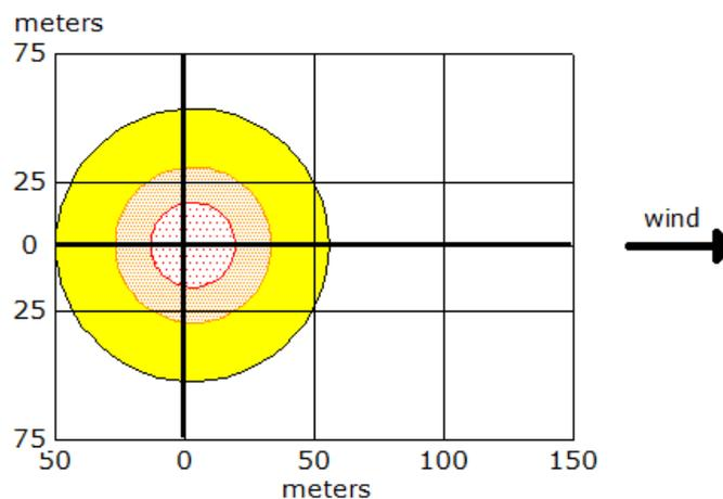
**Figure 10.2: Thermal radiation from jet fire**
