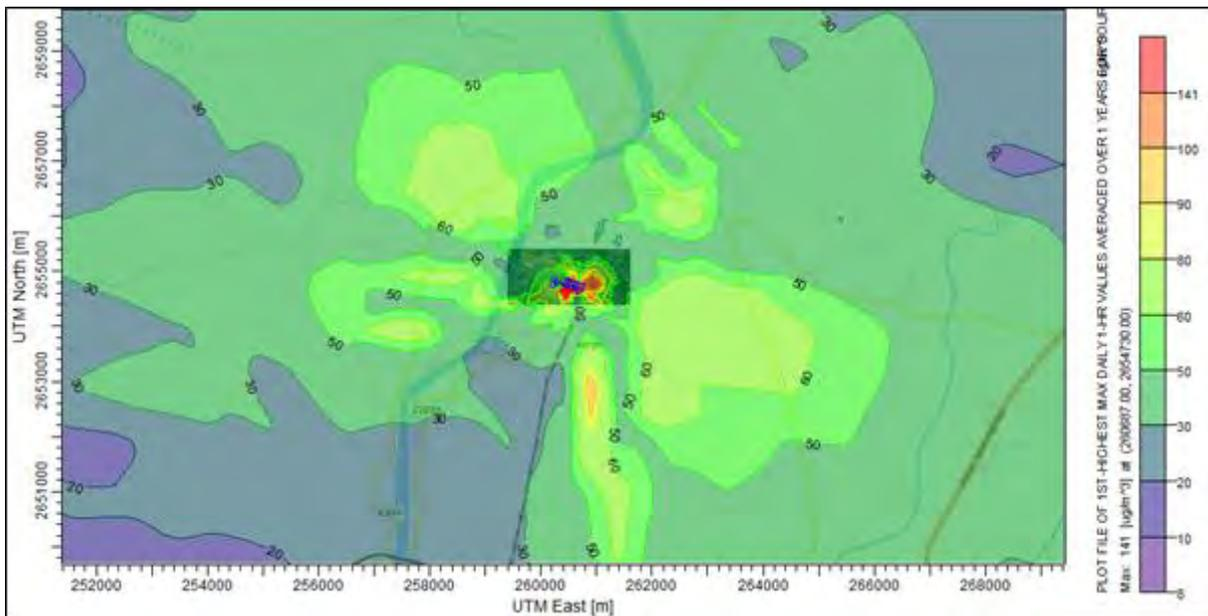
**Figure 7.16: Predicted maximum GLC of NO<sub>2</sub> for 1-Hr**
