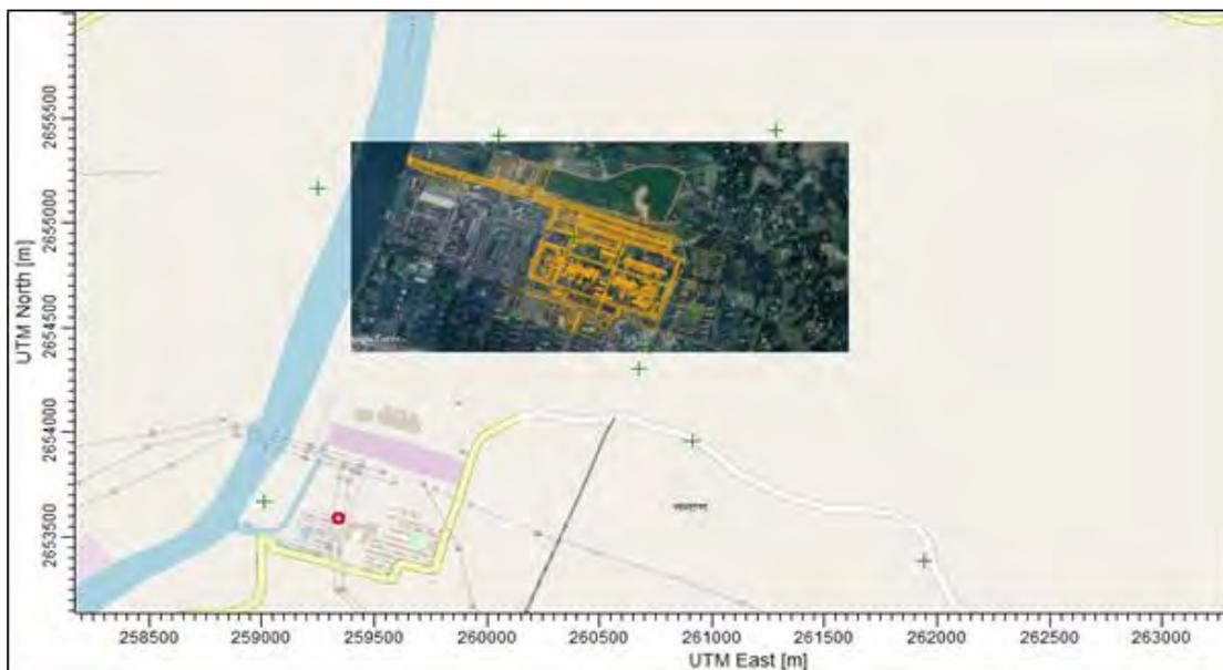
Figure 7.13: Discrete receptors (+) within 5 km around the project site
