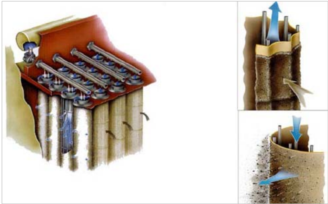
Figure 2-10 Principal function of bag filter and pulse-jet on-line cleaning
