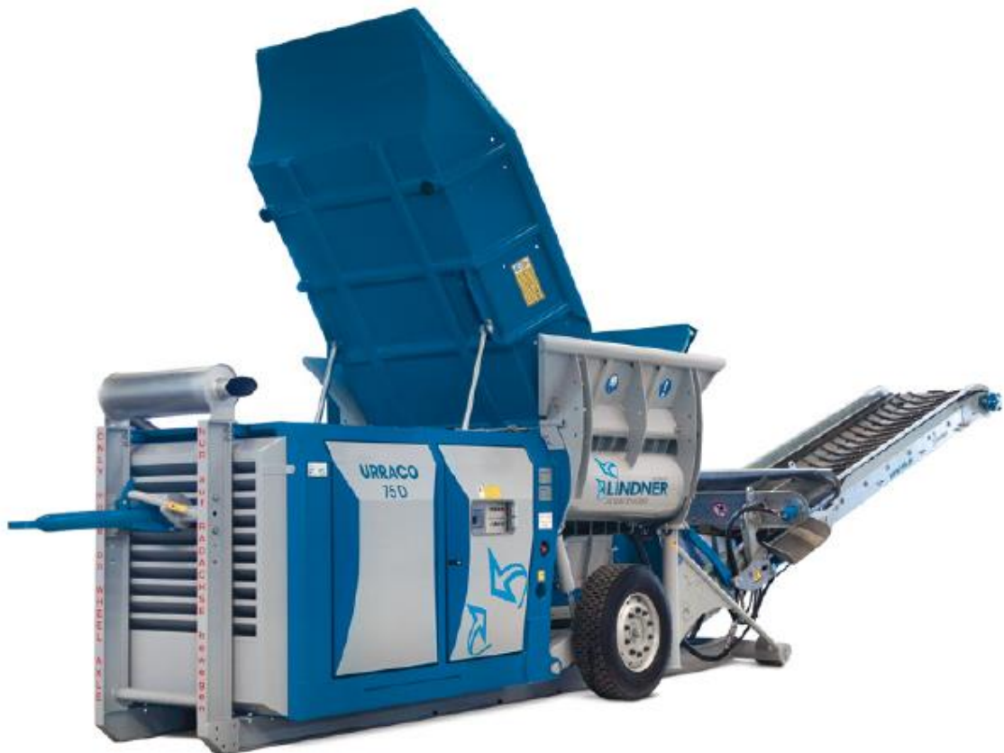
Figure 4-11 Two Shaft Mobile Waste Shredder
