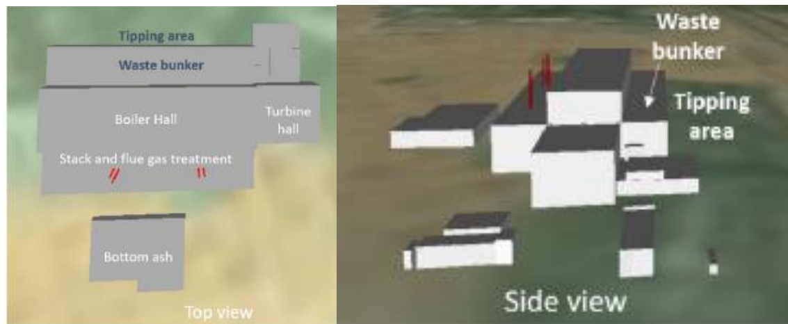
Figure 6-22 Waste bunker and tipping area locations
