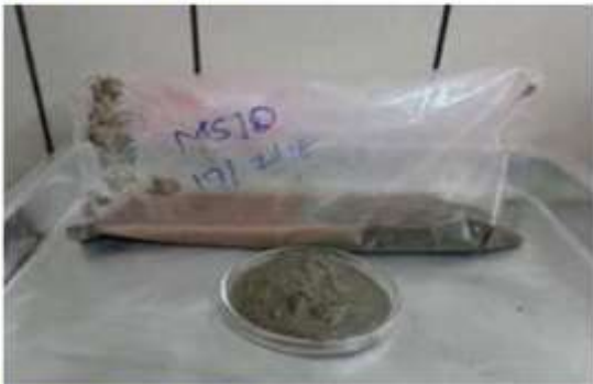
Sediment Sample at MS 10 - Fine sand; broken shells
