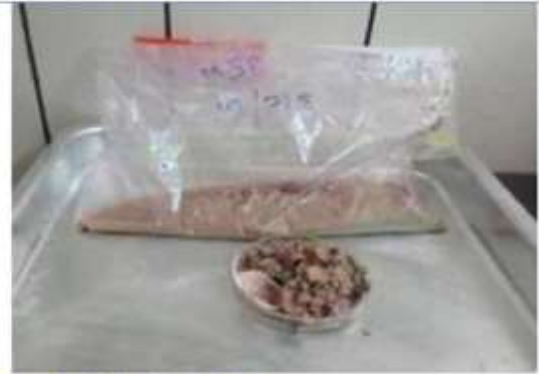
Sediment Sample at MS 8 - Coarse sand with broken shells
