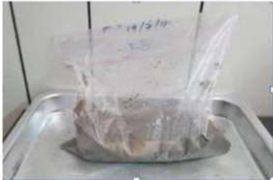
Sediment Sample at MS 9 - Silty sand plus shells
