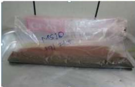
Sediment Sample at MS 10 - Fine sand; broken shells
