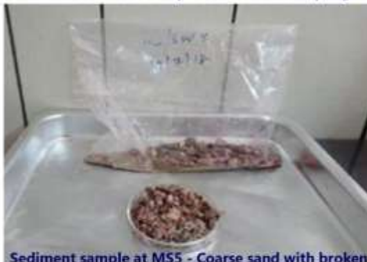
Sediment sample at MSS - Coarse sand with broken shells
