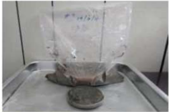
Sediment Sample at MS 9 - Silty sand plus shells
