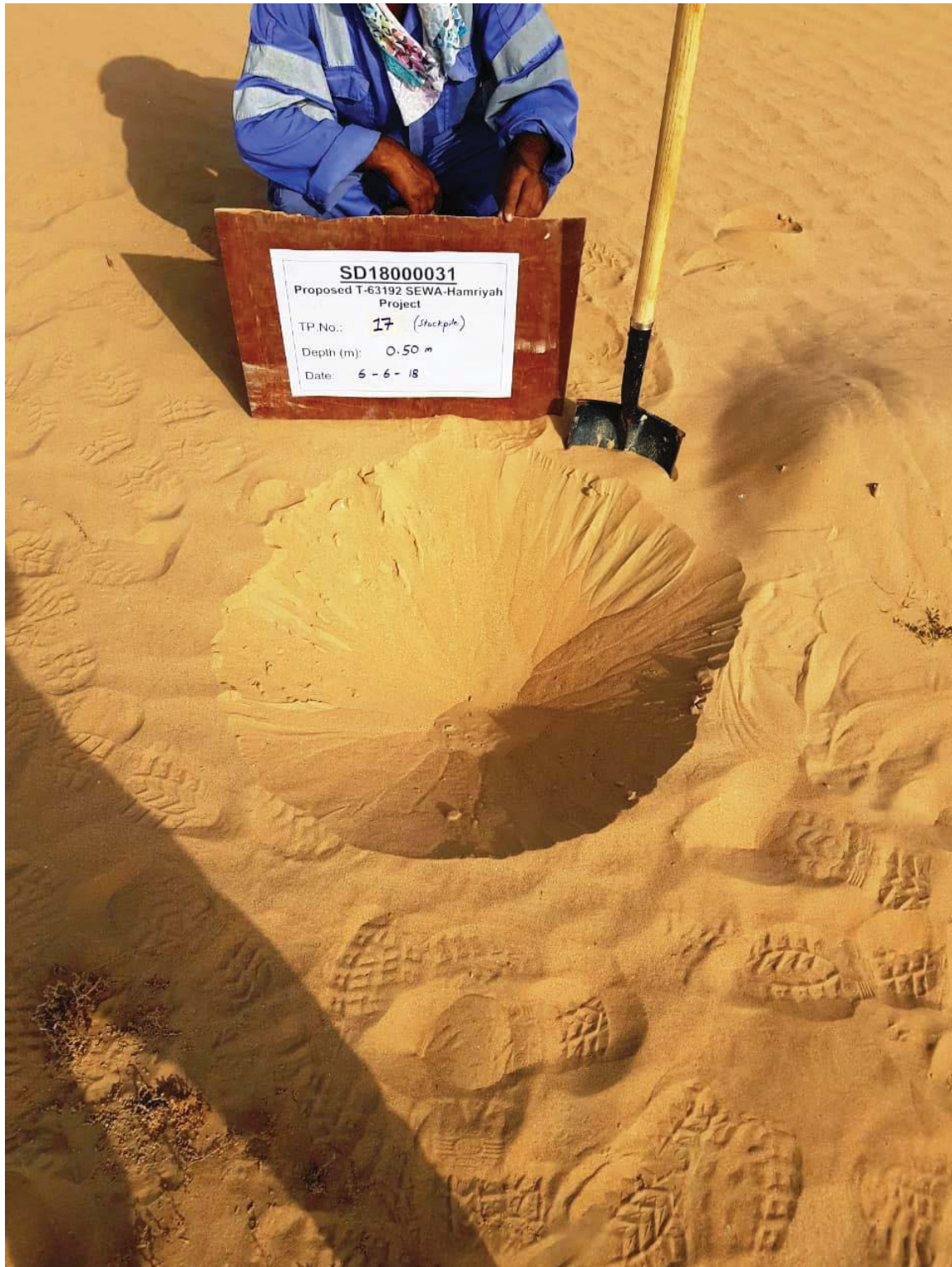
TP: 17 Stock Pile, Depth: 0.00 – 0.50m
