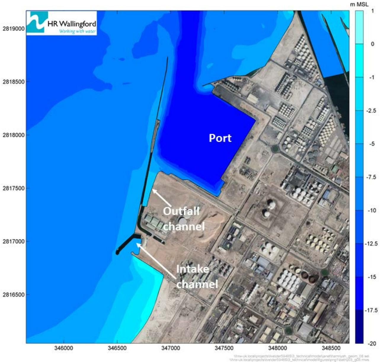
Figure 3.4: Model bathymetry close to the plant
