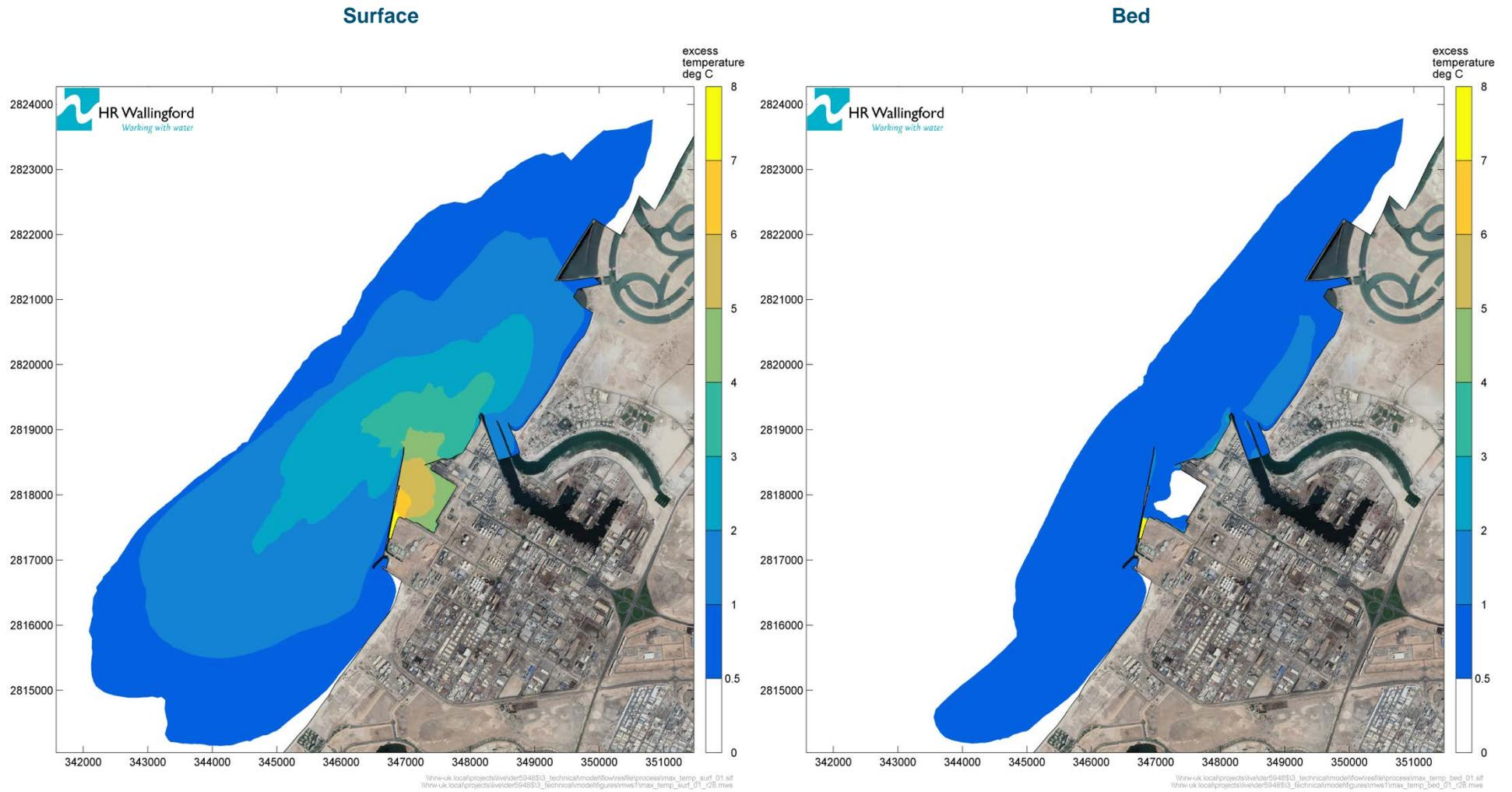
Figure 4.6: Maximum predicted surface and bed temperature with weaker wind, summer Scenario 2
