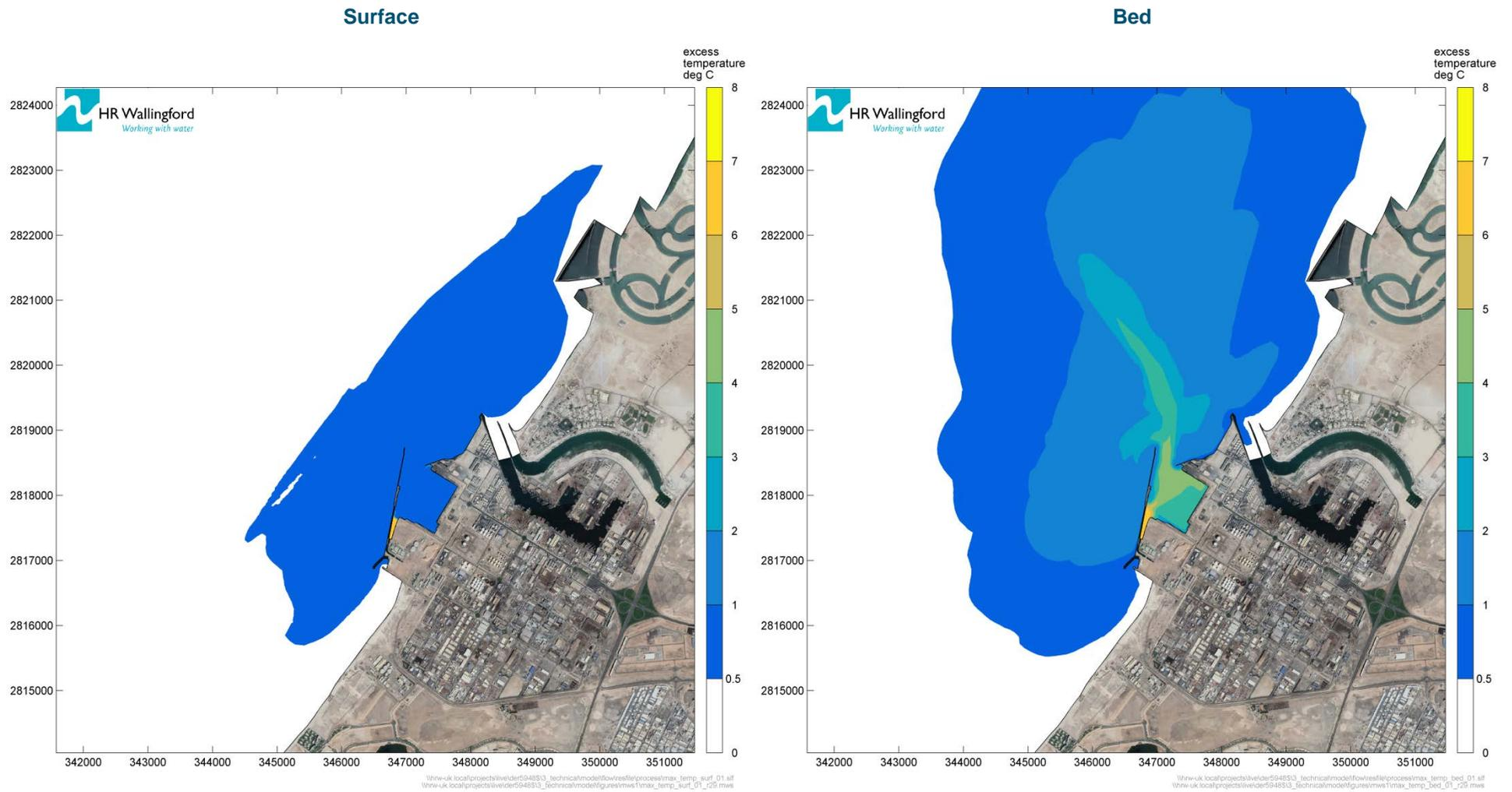
Figure 4.8: Maximum predicted surface and bed temperature with weaker wind, summer Scenario 3
