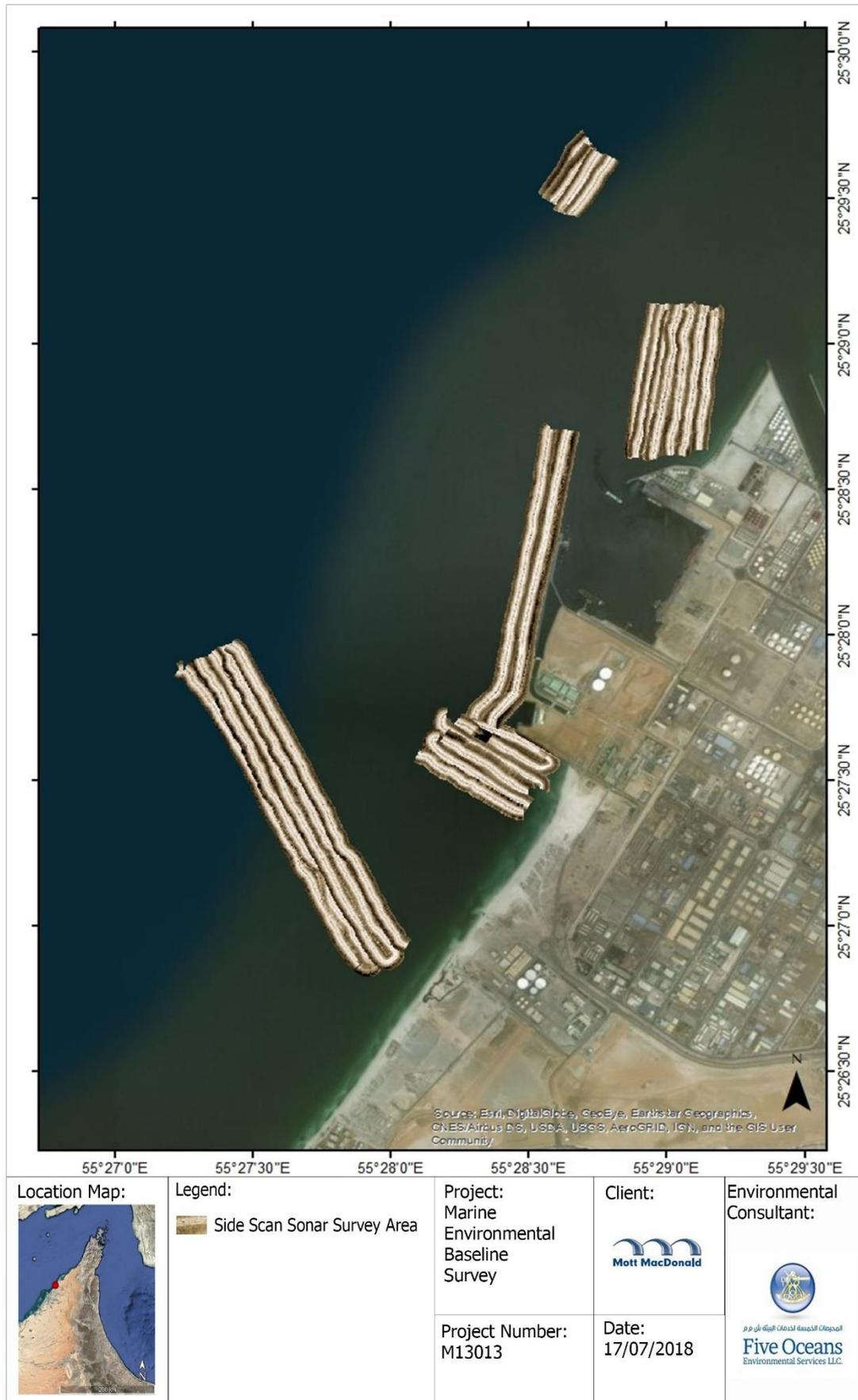
**Figure 4.5.3: Extent of side scan sonar coverage**
