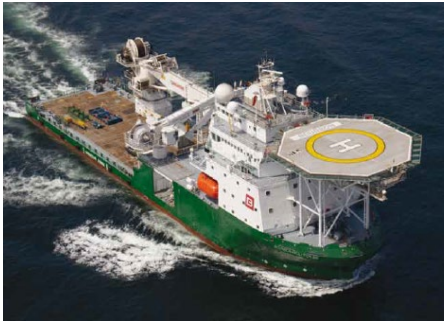
Figure 4.9: Typical installation vessel
