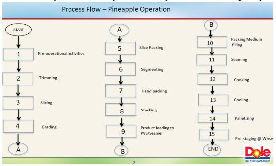
Figure 2.2-1: Process Flow Chart for Pineapple Processing
